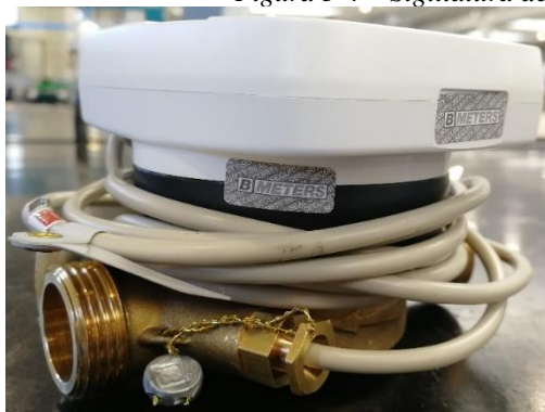
Figure 3-4- Heat meter sealing after positive initial verification
