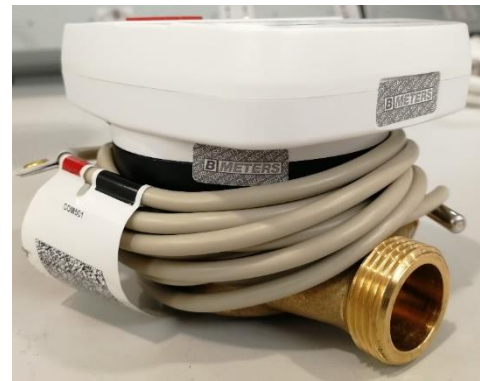
Figure 3-4- Heat meter sealing after positive initial verification
